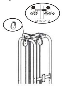
Figure 4. Bolt on the teardrop pulley.
